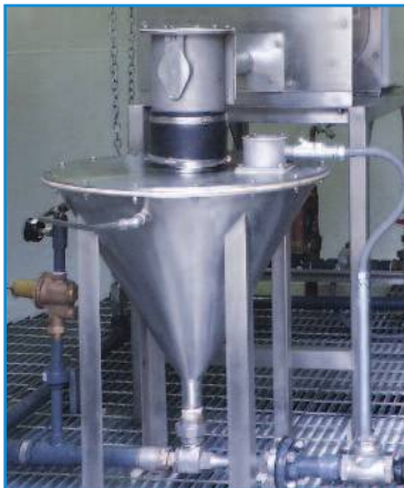
A Model W-105Z Volumetric Feeder metering into a high capacity Wetting Cone.
