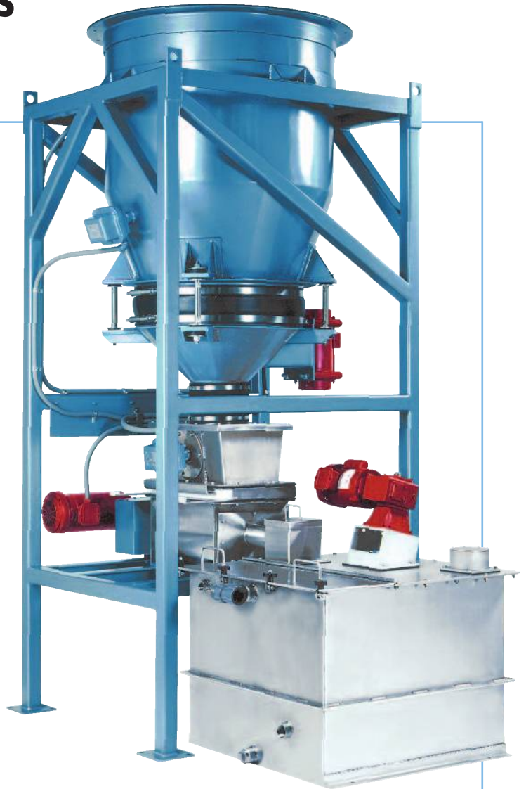
A Model W-105Z Volumetric Feeder mounted beneath a 50 cubic foot Storage Bin equipped with a Vibrating Bin Discharger and Level Probes. The Feeder discharges into a 200 gallon Dissolving Tank.
