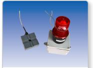
Sensor mounts in spill containment basin. The sensor utilizes a phototransistor to detect spills and activate a relay switch which triggers light to alert workers.
