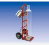
Portable electronic scale with a 4-20mA output, NEMA 4X indicator box and coated steel hand cart. Optional battery. Capacity to 349 lbs.
