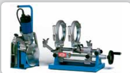
Maxiplast Butt Fusion Welder with contact heating element – PE, PP, PP-RCT, PVDF, ECTFE
