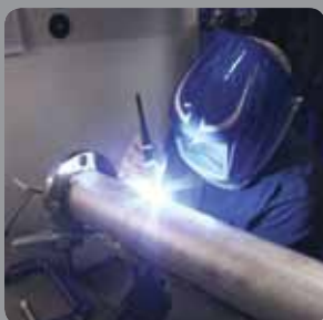
TIG Welding for fabrication of shaft extensions
